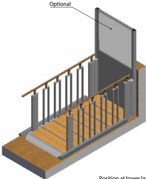
Position at lower landing
